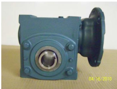
400-02612 Reducer, Morse, 206Q56H15 Through Style, Pin Feeder Drive
